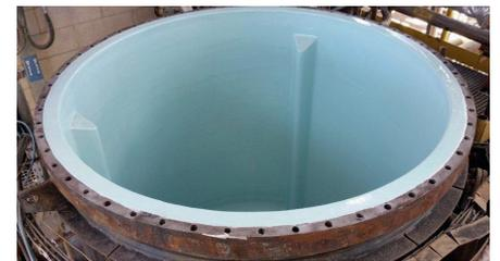
The light colours of Belzona 1593 allow easy visual inspection in vessels.
